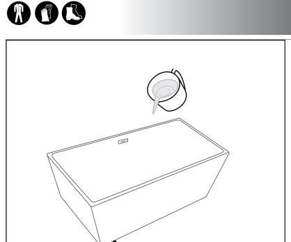
Pour some water into the bathtub to test drainage and check for leaks. If necessary, adjust by legs by tightening with a spanner wrench. If a leak is found, adjust bathtub to level. Adjust the feet screws and make sure the water flows into the drain.
