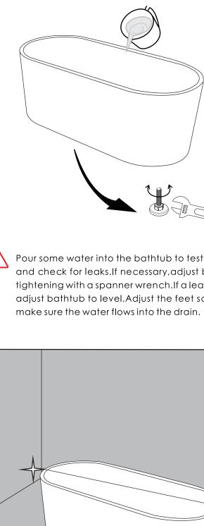
Pour some water into the bathtub to test drainage and check for leaks. If necessary, adjust by legs by tightening with a spanner wrench. If a leak is found, adjust bathtub to level.Adjust the feet screws and
