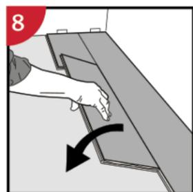
8 Second plank, second row: Place the plank close to the short end of the previous plank and fold it down in a single action movement. Push it down so it engages the first plank and clicks tightly together. Use a rubber hammer along the short end.
